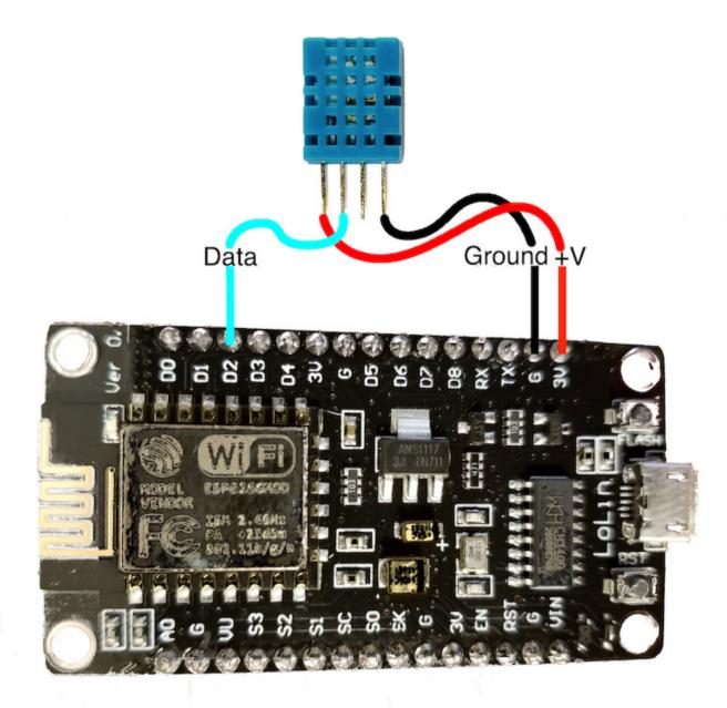
If you have a DHT mounted on a module then you need to check the pinout, usually indicated on the board, with + (to 3V pin), - (to G pin) and **out** or **data** (to D2 pin):
